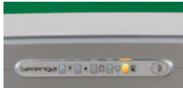
Amber LED indicates a fault.
