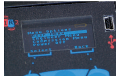
IR2-TESTWARE™ handset includes OLED screen
