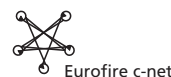
Illustration: Network of Eurofire panels, in star format [wired to the CAN network facility]
