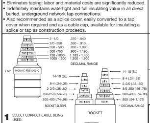
**CUT OFF ROCKET SLEEVE** AND CAP AT TIP OF ARROW LEAVING CORRECT CABLE SIZE SHOWING ON OPENED ROCKET AND CAP.
