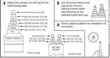
Apply silicone grease. Slide cut rocket and cap over prepared cable.
