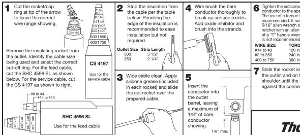
Tighten the setscrews down on the conductor to the specified torque. The use of a torque wrench is recommended. If not available, use a 5/16" allen wrench or a 3/8" drive ratchet with an allen adapter. The use of a "T" handle wrench or 1/2" drive is not recommended.
