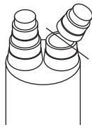
Select correct cut-off ring on tower for wire being used. Cut off end of tower at the tip of arrow, leaving the correct wire size showing.
