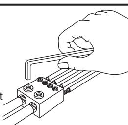
Insert conductors into connector. Tighten down Set Screws to recommended torque. Mate two halves of "Flood-Seal"® Housing for a watertight fully insulated connection.
