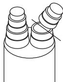
Select correct cut-off ring on tower for wire being used. Cut off end of tower at the tip of arrow, leaving the correct wire size showing.
