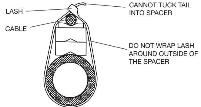
\*\*THIS METHOD OF INSTALLATION WILL NOT SECURELY FASTEN THE SPACERS TO THE ASSEMBLY.
