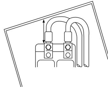
6. Strip insulation to length of compression barrel as shown in table in column "A" to permit full insertion of wire. Scratch brush the aluminum conductor before installation. Select appropriate tool and dies as shown in the table, and make the required number of crimps.
