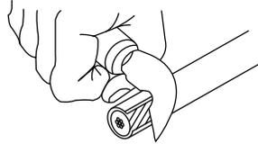
3. Remove oxide film with wire brush from the stripped portion of the conductor.
