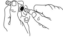
5. Use circumferential or hex dies. Compress from base of socket toward cable. Remove flash. Remove excess inhibitor before slipping the insulating sleeve into place.
