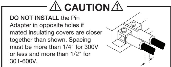
4. Check wiring room leading to the mechanical equipment lug to be sure use of the Pin Adapter will not reduce the minimum wire bending space required by Table 312.6(A) of the National Electrical Code\*\*. (Measured without cover installed as shown in Step 5). \*\*Registered trademark of the National Fire Protection Association.
