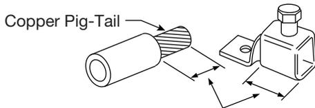
3. Check diameter of mated insulating cover to assure that there is no interference in any direction when it is installed
