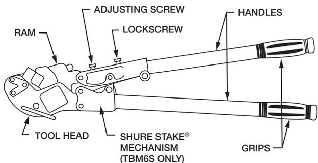
SHURE STAKE® MECHANISM IS DESIGNED TO PROVIDE COMPLETE CLOSURE.
