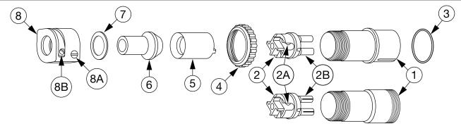
\*NOTE: Hand assemble <u>both</u> cable clamp yokes (#8B), and <u>both</u> machine screws and nuts (supplied loose) onto cable gland nut #8 as shown. Alternately tighten screws to firmly grip cable & bushing to 10-15 in-lbs. Use of power tools is NOT recommended unless verified torque limit <15 in-lbs.
