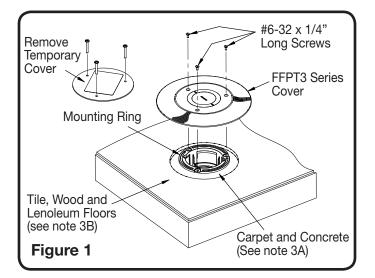
After cover is screwed to Poke-Through, push down on top to fully seat cover to floor.
