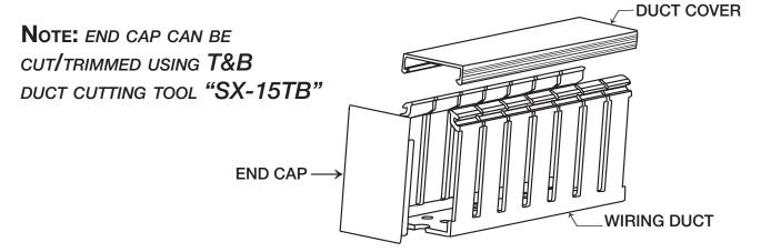
STEP 3: INSTALL END CAP TO DUCT. LEGS OF END CAP WILL ALIGN WITH SIDE WALLS OR FINGERS OF DUCT.
