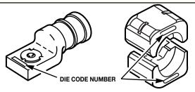
Select appropriate installing die by matching the hydraulic head die code number to the connector's die code number.
