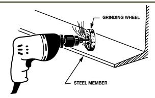
Remove paint, scale, or other foreign matter from the structural member to which the ground connector is to be clamped.
