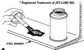
Apply a thin layer of T&B's KOPR-SHIELD® Compound onto the cleaned structural steel member.
