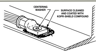
Place the flat surface of connector tongue onto the treated structural steel member. Centering washer should be as shown.
