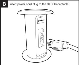
**IMPORTANT:** Press the TEST button (then RESET Button) every month to assure proper operation.
