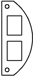
FPT4-CPB-2KEY T&B KEYSTONE HUBBLE LEVITON-QUICKPORT (2) SHIPPED WITH POKE THROUGH BASE UNIT CAT. NO. FPT4-8C-C
