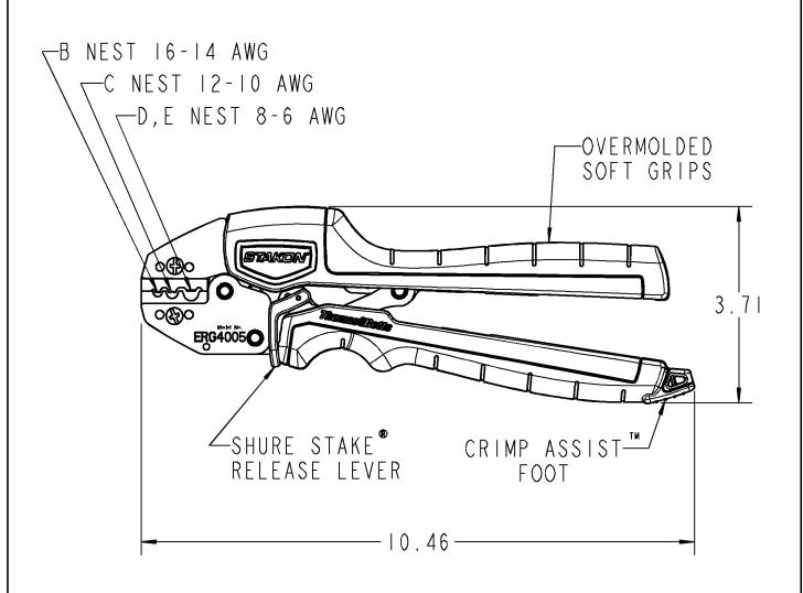
CAUTION: HANDLES NON-INSULATING, DO NOT CRIMP ENERGIZED WIRES
