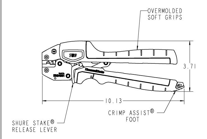
CAUTION: HANDLES NON-INSULATING, DO NOT CRIMP ENERGIZED WIRES
