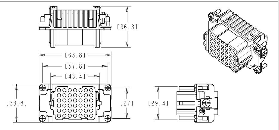
DD-SERIES 10A AT 600VAC: FEMALE INSERT FOR 42 CONTACTS + GROUND GLASS-FILLED THERMOPLASTIC INSERT RATED FOR -40 TO 125°C WITH UL940V-0 FLAMMABILITY RATING CONTACTS MADE FROM SOLID DRILLED COPPER ALLOY WITH HARD SILVER PLATING - HARD GOLD PLATING IS AVAILABLE SCREW TERMINALS FOR USE WITH WIRE RANGE .14-2.5 mm<sup>2</sup> [26-14 AWG]
