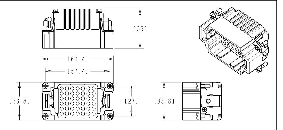
DD-SERIES 10A AT 600VAC: MALE INSERT FOR 42 CONTACTS + GROUND GLASS-FILLED THERMOPLASTIC INSERT RATED FOR -40 TO 125°C WITH UL940V-0 FLAMMABILITY RATING CONTACTS MADE FROM SOLID DRILLED COPPER ALLOY WITH HARD SILVER PLATING - HARD GOLD PLATING IS AVAILABLE SCREW TERMINALS FOR USE WITH WIRE RANGE .14-2.5 mm<sup>2</sup> [26-14 AWG]
