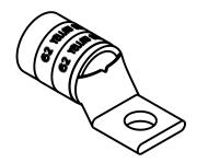
WIRE SIZE: 300 MCM, 4/0 WELD, 650/24 MATERIAL: HIGH CONDUCTIVITY COPPER
