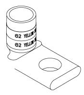
WIRE SIZE: 300 MCM, 4/0 WELD, 650/24 MATERIAL: HIGH CONDUCTIVITY COPPER FINISH: TIN PLATED
