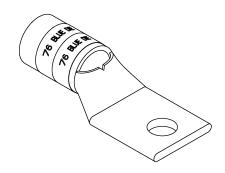
WIRE SIZE: 400 MCM MATERIAL: HIGH CONDUCTIVITY COPPER FINISH: TIN PLATED
