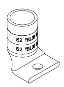
WIRE SIZE: 300 MCM, 4/0 WELD, 650/24 MATERIAL: HIGH CONDUCTIVITY COPPER
