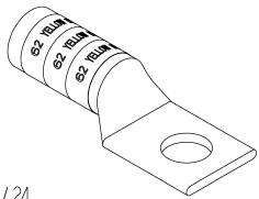
WIRE SIZE: 300 MCM, 4/0 WELD, 650/24 MATERIAL: HIGH CONDUCTIVITY COPPER FINISH: TIN PLATED
