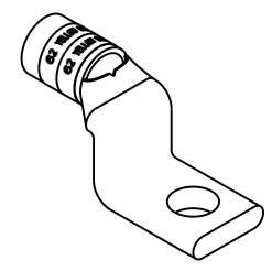
WIRE SIZE: 300 MCM, 4/0 WELD, 650/24 MATERIAL: HIGH CONDUCTIVITY COPPER
