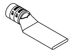
WIRE SIZE: 350 WELD, 400 WELD, 500 MCM MATERIAL: HIGH CONDUCTIVITY COPPER
