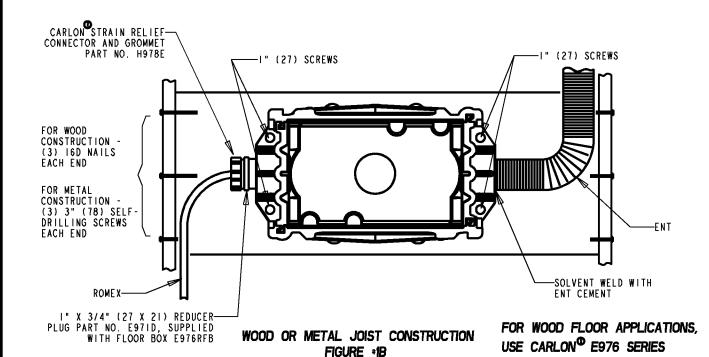
INSTRUCTIONS FOR CARLON RECTANGULAR FLOOR BOX PART NO. E976RFB FOR USE IN FRAME CONSTRUCTION
